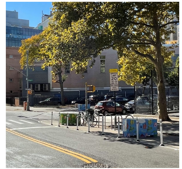
Restricting parking near corners using physical interventions like markings, plastic delineators, concrete blocks, bike parking, etc.
